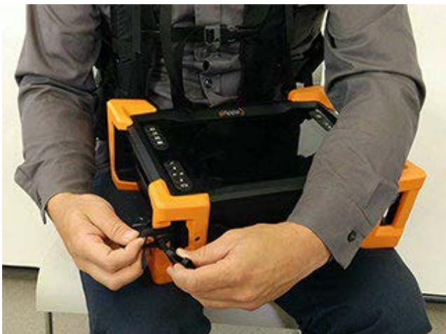
Figure A-9 Securing anchor strap
