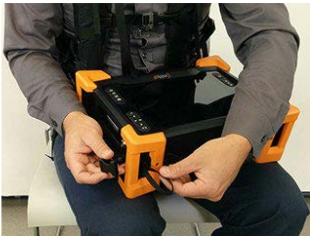
Figure A-8 Sliding strap loop through bumper hook
