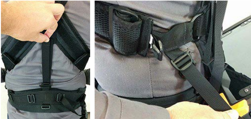
Figure A-3 Adjusting the belt's height
