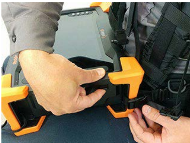
Figure A-14 Closing battery compartment door.
