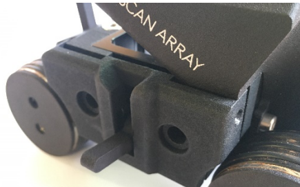
Figure 20: Prising off the right side cover
