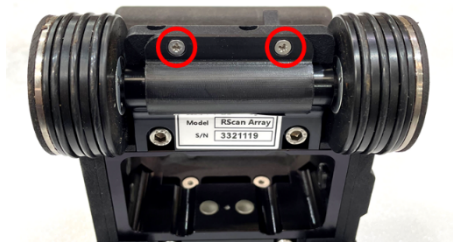
Figure 14: Rear fairing dust cover screw location
