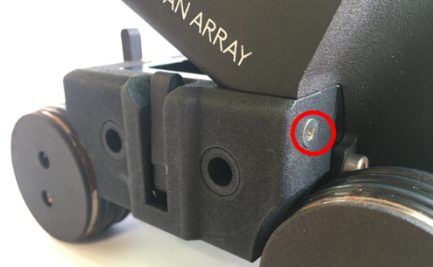
Figure 19: Right-side cover front bolt location
