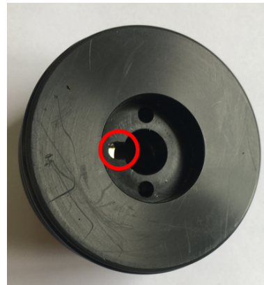
Figure 32: Inside face of wheel keyway location
