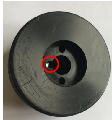
Figure 29: Inside face of wheel keyway location
